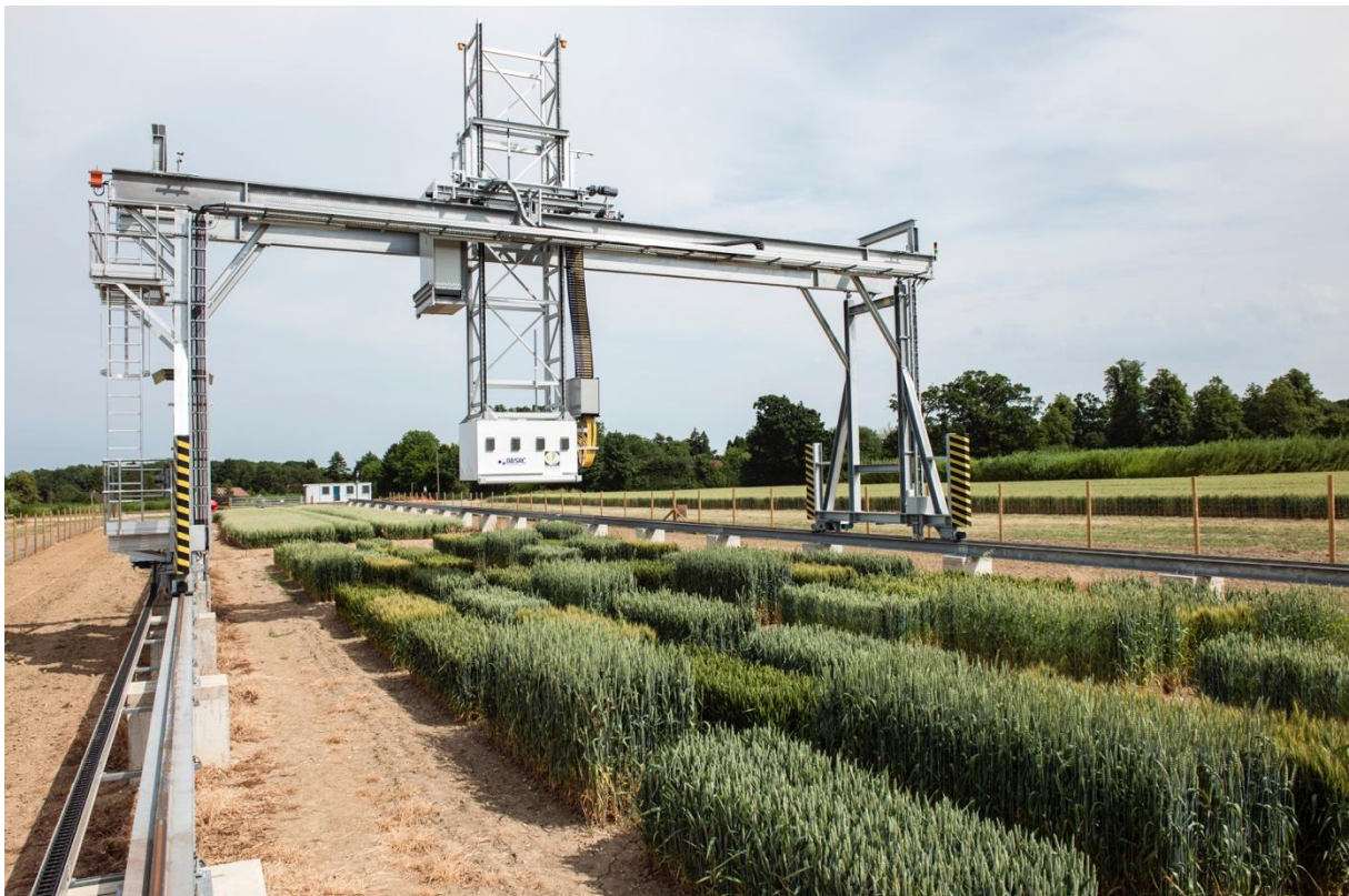
Figure 1. The Rothamsted Field Scanalyzer. A purpose built autonomous platform for spatially and temporally intensive monitoring of field trials.
